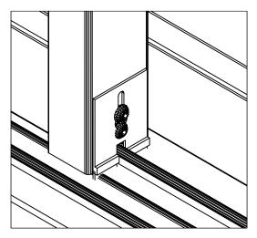
19. Optional: Add bug sweeps at bottom ends of interlocks at interior and exterior. To install back out bottom panel screw 2-3 turns or enough to slip bug sweep over and under screw head. Adjust and then tighten screw.
