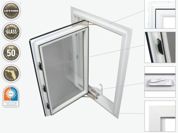
Sturdy Construction Multi-chamber construction improves strength and thermal performance. Fusion-welded corners add strength and prevent air/water infiltration.
