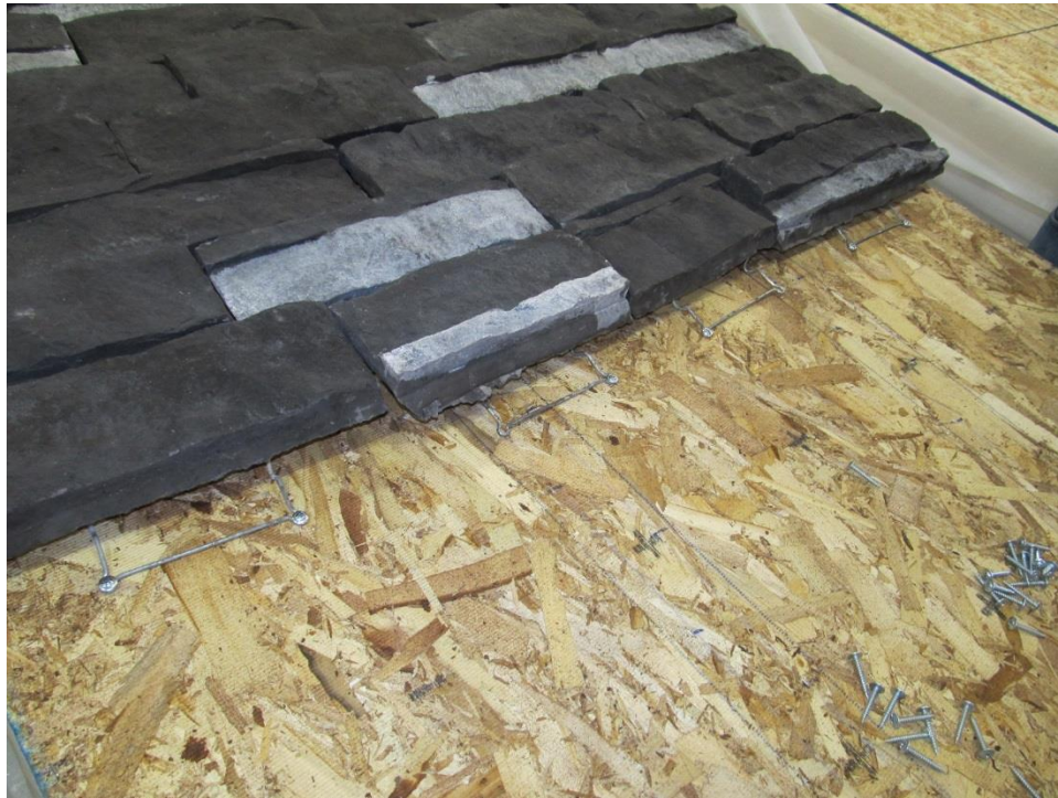
Figure 6: Attaching ClipStone to a Specimen
