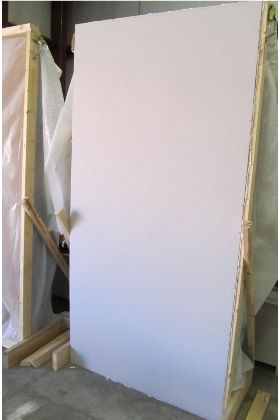
Figure 13: Interior Sheathing (Gypsum) Attachment
