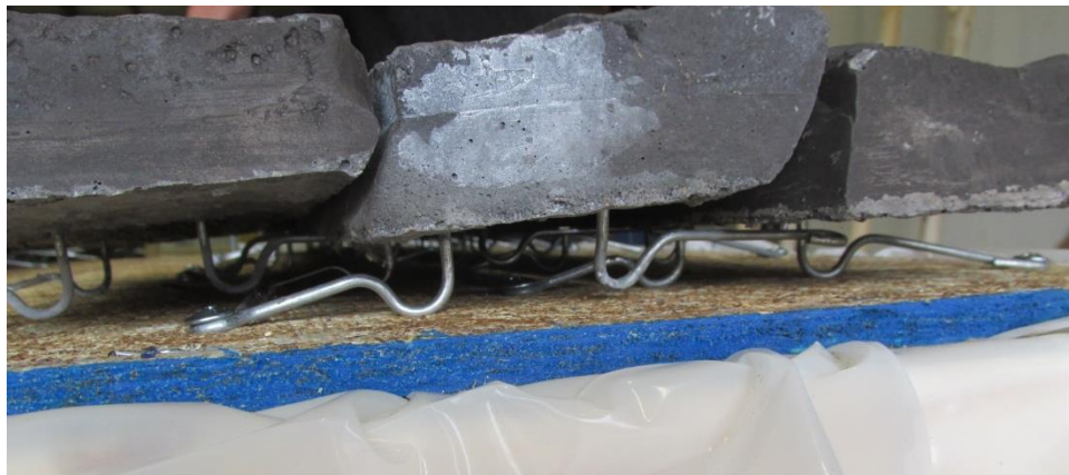
Figure 9: Edge View of ClipStone Attachment
