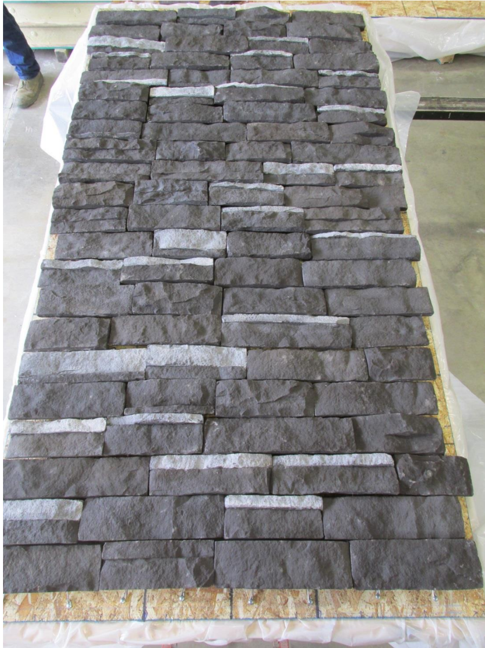
Figure 11: A Specimen after Finish of ClipStone Attachment
