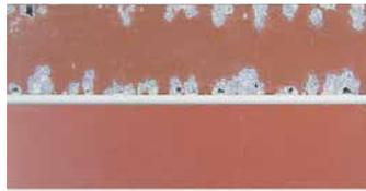
(TOP) SINGLE-COAT POLYESTER OVER METAL FROM A SCRAP-BASED MINI-MILL
