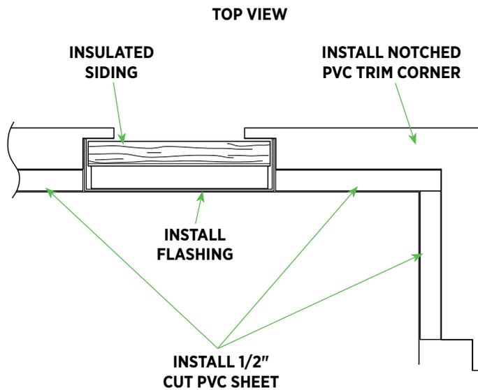
Because insulated siding is approximately 1-1/4" thick, you'll need to pack out trim boards to create a pocket for the siding.
