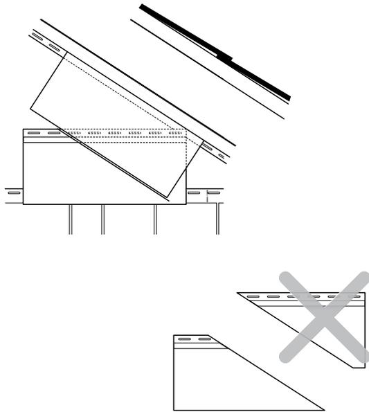
Cedar Discovery Half-Rounds can be locked directly onto other Cedar Discovery panels. If desired for transitions, panels can be installed using starter strip (CDSS) over drip cap, or into T-Channel or lineals.
