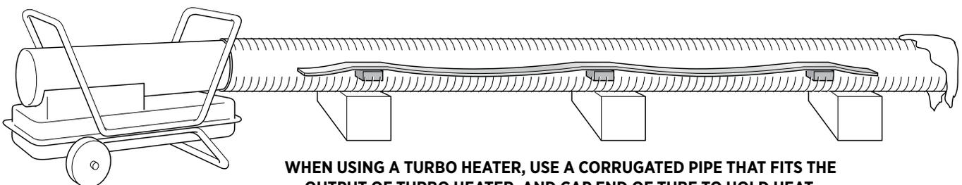
**WHEN USING A TURBO HEATER, USE A CORRUGATED PIPE THAT FITS THE OUTPUT OF TURBO HEATER, AND CAP END OF TUBE TO HOLD HEAT.**
