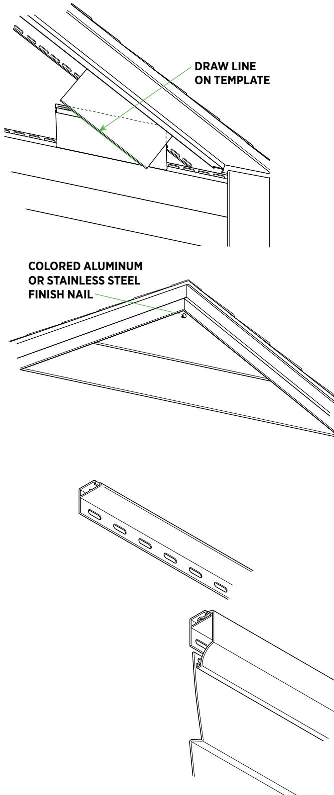
**Note:** All soffit accessories must be installed before gables are installed.
