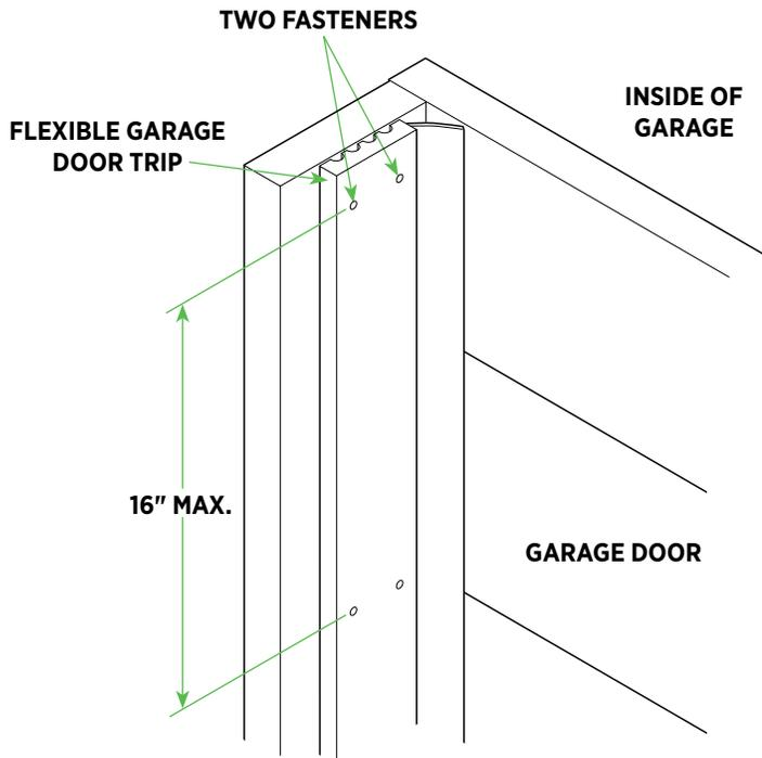
**Note:** Apply 2 fasteners per width of product, fastening no more than 16" vertically as well.
