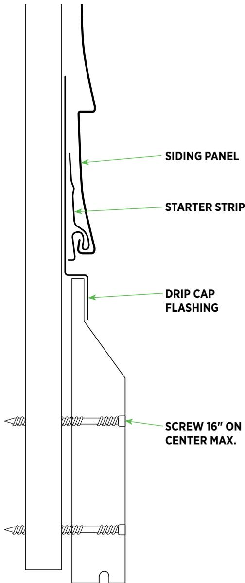
Skirt or frieze boards can make an attractive band at the bottom of walls with the application of any siding panels. Use a flat PVC trim of any size as a frieze option.
