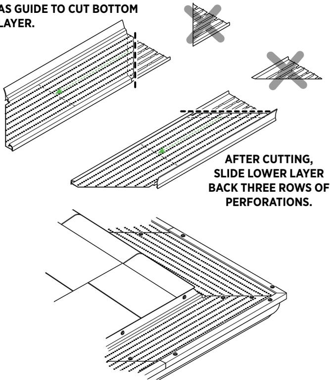
AFTER CUTTING, SLIDE LOWER LAYER BACK THREE ROWS OF PERFORATIONS.
