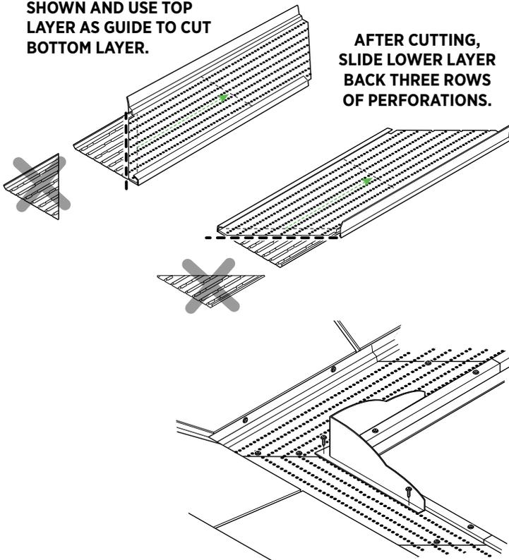
AFTER CUTTING, SLIDE LOWER LAYER BACK THREE ROWS OF PERFORATIONS.
