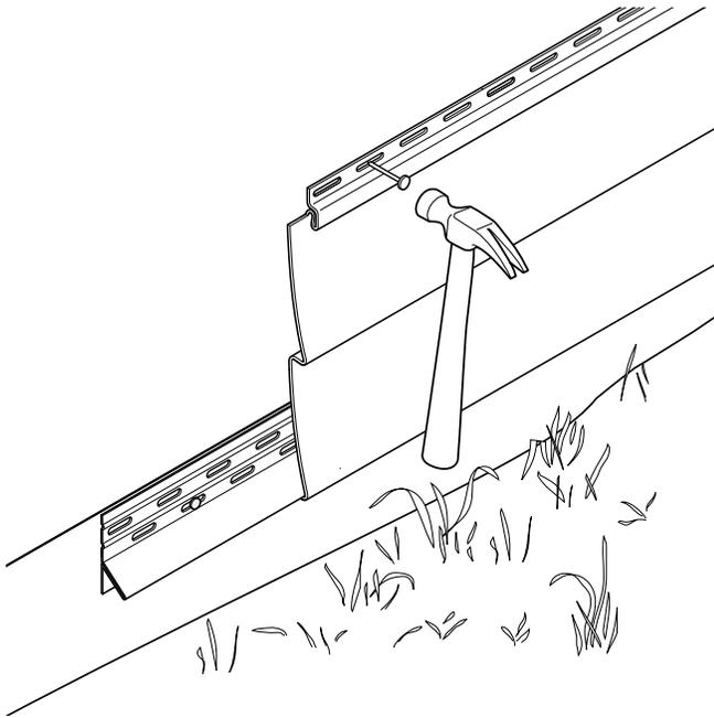
**Note:** A 6" minimum clearance should be given between ground and bottom of the first row. If there is a wave in the wall, use shims to straighten out the wall. This will help to smooth out uneven surfaces.
