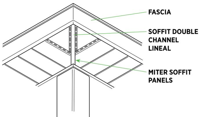
Enclosed eaves are typical of re-siding projects. Installing soffit over enclosed eaves is almost identical to the process used for open eaves. J-Channel or F-Channel can be used to receive soffit panels.
