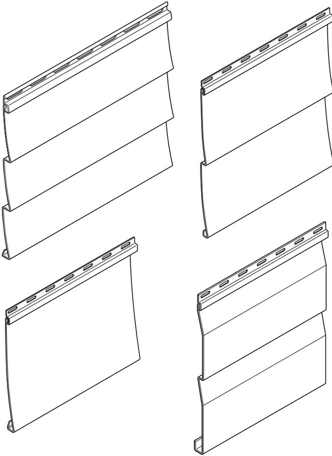
Vinyl siding comes in many shapes, textures, and colors, creating a wide array of looks. It comes in panels that can be installed horizontally or vertically.
