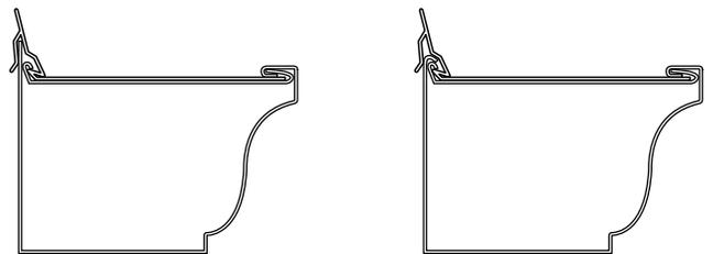
**Note:** To cut the DuoPro continuous hanger to receive downspout from above, secure the two layers of the product together with 1/2" screws before cutting for the 2nd floor downspout connection.
