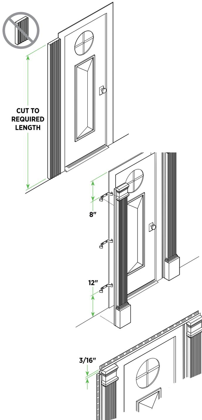
**Note:** Pilasters are available in 96" and 144" lengths. Pilaster package includes: two pilasters, clips, two caps, two bases and screws.
