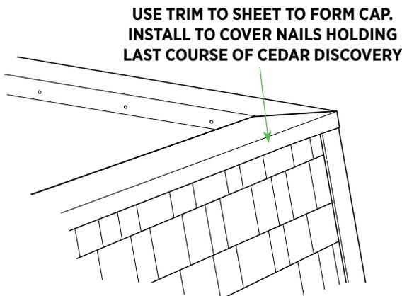
Install all Cedar Discovery courses, cutting the last course as required. Cut nail slots and nail into top of mansard following standard installation guidelines for last course of panel being used.
