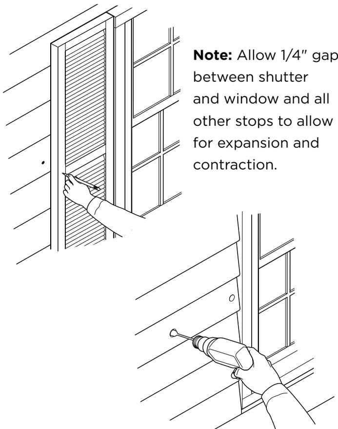
**Note:** Allow 1/4" gap between shutter and window and all other stops to allow for expansion and contraction.
