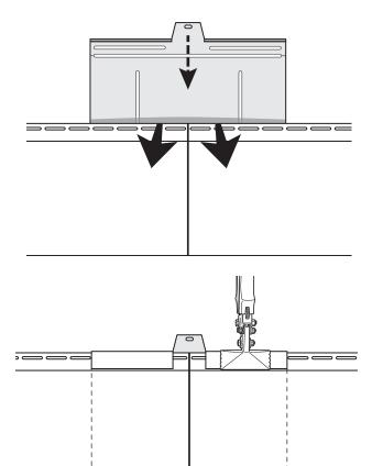
• Finish nailing both Mastic EverPlank panels into place starting with the first fully exposed nail slot on either side of the bonding plate and then with nails every 16". Stop nailing 36" from the next seam to allow the installation of the next bonding plate in the same manner as outlined above.
