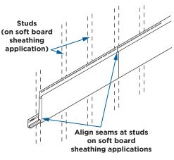
Panels must butt together at stud location. Firmly lock on starter strip or course below. Butt panels at ends. Fasten every 16". Stop fastening 36" from seam to be bonded to allow room for Bonding Plate to slide in.
