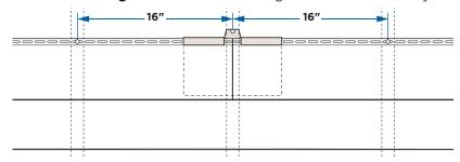
Nail base sheathing: fasten through slots next to Bonding Plate and every 16".
