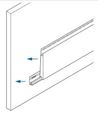
Install on solid nail base sheathing, such as plywood or OSB, or over soft board sheathing with studs every 16" on center. A water resistive barrier (WRB) is necessary for a proper and secure installation.
