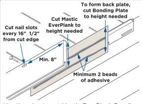
Use tin snips to cut Mastic EverPlank Bonding Plate to height needed to rest in the channel of the previous course.
