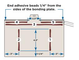
**Purge adhesive** per installation instructions and apply properly mixed adhesive in order shown.
