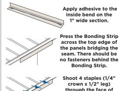
shoot 4 staples (1/4" crown x 1/2" leg) through the face of the bonding strip and into the panels. Do not overdrive the staples.
