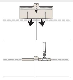
Insert and slide Bonding Plate panel down into starter strip or top lock of course below. Bend tabs and crimp firmly using a 3" hand seamer.
