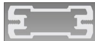
(1) Aluminum mill structural tube mull
