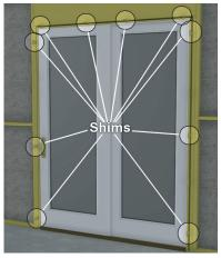
(1.L) (Recommended) The door should slide open / closed, and lock / unlock without binding. If not, the sliding door needs to be squared by adjusting the roller sets along the bottom of the door. Locate the roller adjusting screws by removing the plastic plugs at the interior lower corners of the door, then use a Phillips-head screw driver to adjust them until the door slides open / closed, and locks / unlocks without binding. Replace the plastic plugs to cover the adjustment screws.
