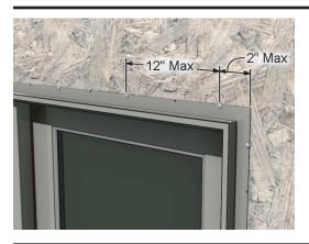
(1.I) (Required) From the interior, you should see a nominal 1/8" gap between the door and frame along any edge. If the gap varies, then the frame is not square. Shim and adjust as needed to achieve a square frame, then complete the nailfin fastening by placing fasteners in the provided nailing fin holes, spaced a maximum of 12" apart and 2" from the ends. Refer to Step 2.C for fastening Transom Gusset Plates.
