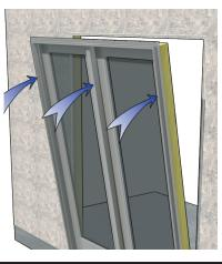
(1.F) (Required) Check the unit to make sure it's plumb and square, then place a few fasteners through the provided nailfin holes, anchoring the unit to the wall.
