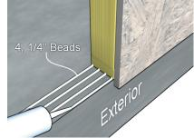
Sill is a representation only. Refer to local building codes for actual opening requirements. (1.D) (Required) Apply a generous continuous bead of sealant (at least <sup>1</sup>/<sub>4</sub>" diameter) along the top and sides of the rough opening exterior to ensure an adequate seal between the back of the nailing
