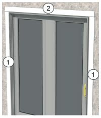
(1.0) (Recommended) Apply a finish material to the interior of the door as soon as possible to keep the wood clean and avoid damage from moisture. Some light sanding may be needed before applying the first coat... always sand WITH the wood grain. Make sure that sandpaper does not touch the glass. NOTE: KEEP FINISH OFF hardware and weather-stripping. Following the instructions provided by the manufacturer of the finish material for best result.
