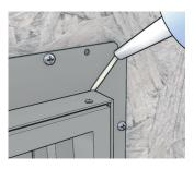
the unit joints (corners and mullions) making sure that none of the joints have gaps or that the sealant is cracked. If there is a visible crack width, use a clear or color-matched 100% silicone and reseal the joint(s). (1.N) (Recommended) Following the flashing manufacturers' recommendations, apply flashing to the nail fins and surrounding wall surface starting with the sides, then the top, creating a shingle effect (see illustration).
