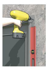
(1.G) (Required) Shim unit snugly, but do not over shim, or force shims, causing the jambs to bow in. NOTE: If the sill is not level, shim low spots beginning at the side jambs. The sill must be level or the doors may bind when opened. If sill shims are needed, go back and make sure there is a full seal between the sill and the subfloor at the interior and exterior edges.
