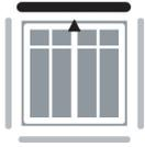
**2a) Preparing the Head Casing** For combination units that have a single width (single windows with single transom) the *head casing* will be precut with opposing 45° angles. These cuts should line up with the miters at the top corners of the window.
