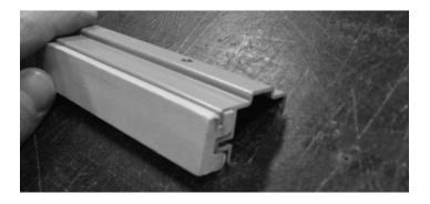
29. Slide the head inside stop assembly in place above the active panels. It may be necessary to adjust the panel rollers to drop the panels to provide clearance for installation. Fasten in place with the #8 x 1" screws in the holes provided. (fasten at the ends first; the center hole will then be accessible by unlocking the active panels and sliding them open. They are now retained by the head inside stop)
