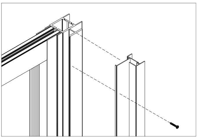
Attach OXO screen jamb (—1) to XX adaptor (—1) by snapping it on. Secure screen jamb with three #7 x 7/16" self drilling screws, one at each end and one the same height as the door latches.
