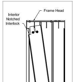
Note: The interior vent will have the interlock notched back at the head and sill. The head end of an XXR or OX configuration is shown in the figure above.
