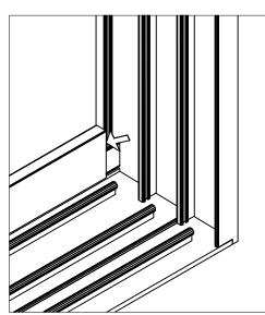
7. If the sill riser is added sealant must be applied from the top of the riser to jamb joint down to the frame sill.
