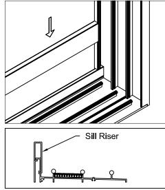
6. If the sill riser is required use a rubber mallet to drive it over the dam of the frame sill.
