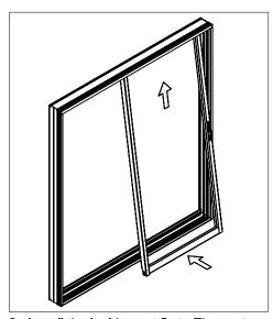
8. Install the inside vent first. The vent installs from the outside. Push the top of the vent up into the head and swing the bottom onto the sill.
