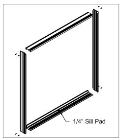
3. Assemble the door frame using the #8 X 1" zinc pan head screws (8).
