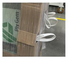
• **Modular packaging:** Frame pieces and door panels are packed and shipped together with the hardware kit and match the bill of materials for a customer's order. Convenient handles make door panels easier to unload and carry
