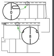
Very important: Align the bottom right end of panel on the even rows with the "EVEN" alignment line on the panel below. Align odd rows with the "ODD" line on the panel below.
