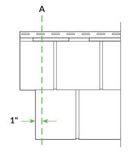
Panels must always be installed from left to right. Cut the first panel of the first course at "A", which is 1" in from the bottom left end of the panel. Allow 1/4" gap at all corner posts, J-Channel, or other stops.
