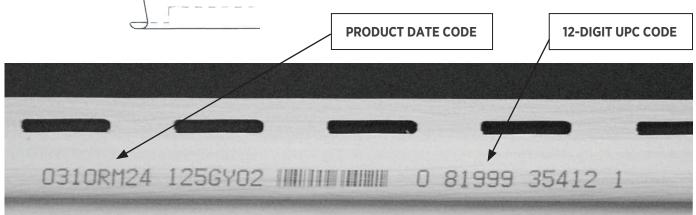
You will have one of two types of Date Codes on your Variform Vinyl Siding, depending on when your siding was manufactured. Products manufactured after 2008 will have an ink-jet printed Date Code on the roll of the top lock (the ink-jetted panels will also include a 12-digit UPC code to identify the product). Products manufactured before 2008 will have an embossed Date Code and no UPC code. After you have located the Date and/or UPC Codes, please record them in full on page 1.
