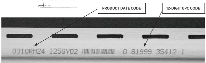
You will have one of two types of Date Codes on your Mastic Vinyl Siding, depending on when your siding was manufactured. Products manufactured after 2008 will have an ink-jet printed Date Code on the roll of the top lock (the ink-jetted panels will also include a 12-digit UPC code to identify the product). Products manufactured before 2008 will have an embossed Date Code and no UPC code. After you have located the Date and/or UPC Codes, please record them in full on page 1.
