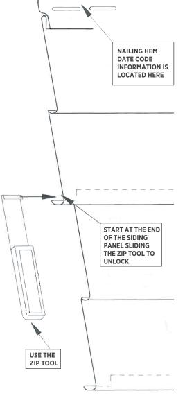
A Date Code is located on the Nailing Hem of all Mastic Vinyl Siding panels. This Date Code provides information that will identify date and time of manufacture, as well as, the specific plant of manufacturer. This information is required to process your claim.
