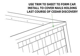
Install all Cedar Discovery courses, cutting the last course as required. Cut nail slots and nail into top of mansard following standard installation guidelines for last course of panel being used.
