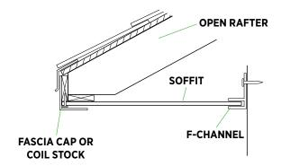
Examine the three illustrations at the left and find one that most closely resembles the construction methods used on your project.
