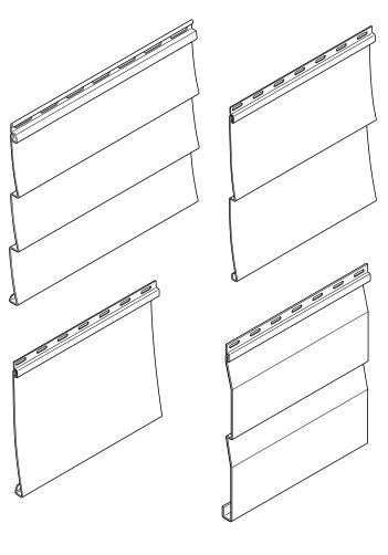
Vinyl siding comes in many shapes, textures, and colors, creating a wide array of looks. It comes in panels that can be installed horizontally or vertically.
