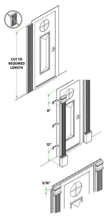
**Note:** Pilasters are available in 96" and 144" lengths. Pilaster package includes: two pilasters, clips, two caps, two bases and screws.
