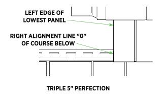
• For Triple 5", align lowest panel left edge with right alignment line "O" of the course below.
