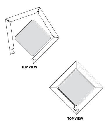
The four-piece design snaps together, requires minimal adhesive and easily fits around existing posts. These post wraps come with a protective peal-away film. Remove this film and corner tape before fastening, painting or adding molding.
