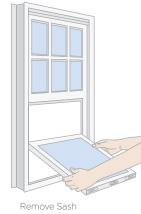
To restore the sash, reverse the procedure above being careful to insert the pin into the balance shoe. Insert the pin on the lower side, then insert the pin on the upper side and straighten the sash back into its level, operating position.
