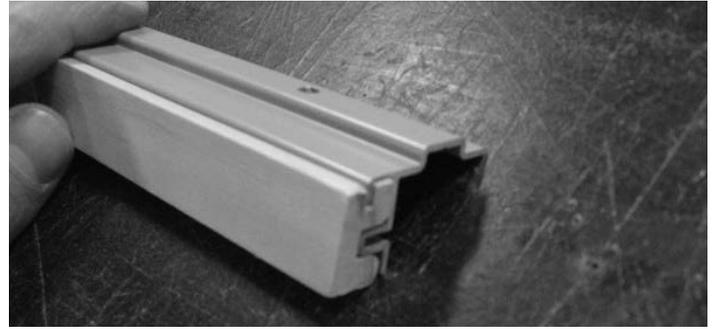
29. Slide the head inside stop assembly in place above the active panels. It may be necessary to adjust the panel rollers to drop the panels to provide clearance for installation. Fasten in place with the #8 x 1" screws in the holes provided. (fasten at the ends first; the center hole will then be accessible by unlocking the active panels and sliding them open. They are now retained by the head inside stop)
