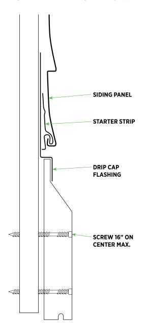
Skirt or frieze boards can make an attractive band at the bottom of walls with the application of any siding panels. Use a flat PVC trim of any size as a frieze option.
