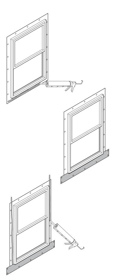
Before installing J-Channel, you must install flashing around windows.
