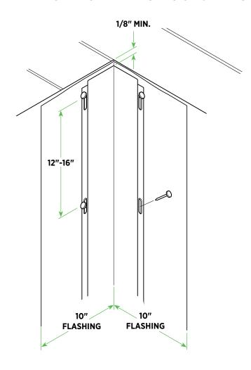
**Note:** These options eliminate the need for exposed fasteners. There are two flanged one piece corner options. One has a solid flange that can be used for any siding type. The second option is not notched and has a flexible hinged nail hem.
