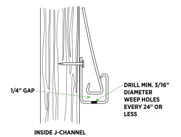
In most situations starter strip is used to start the first course of siding. Special circumstances (panel application around decking, special roof lines and other unique applications) may require other techniques to secure the first panel locking leg. This can be J-Channel or utility trim. In these applications, make sure to leave a 1/4" gap into the J-Channel or utility trim.
