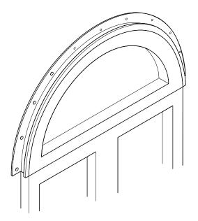
J-Channel is designed to receive the siding and must be installed around all windows, doors, other openings and in the gables and eaves where built-in J-Channel is not present. Install J-Channel in this order: bottom, sides
