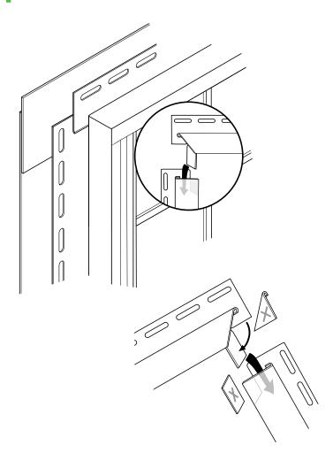
J-Channel is designed to receive the siding panels and must be installed around all windows, doors, other large openings, and in the gables and eaves where built-in J-Channel are not present. J-Channel can be installed over old wood casing leaving the old window casing exposed.
