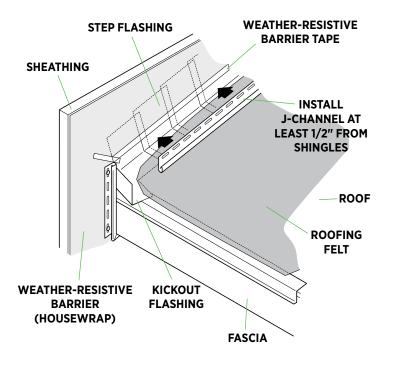
As an alternative to the diverter, create a "kickout" from metal flashing.
