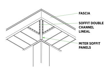
Enclosed eaves are typical of re-siding projects. Installing soffit over enclosed eaves is almost identical to the process used for open eaves. J-Channel or F-Channel can be used to receive soffit panels.
