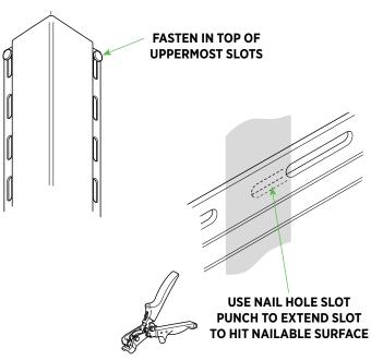
Vinyl siding can expand and contract 1/2" or more over a 12'6" length during normal, yearround changes in temperature. Whether using a nail, screw, or staple to fasten the siding, the following basic rules must be followed:
