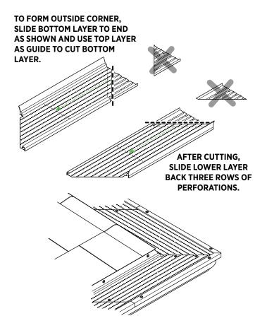
**Note:** Use the DuoPro Access/Corner Kit (UA11500). Ensure prefabricated corner overlaps continuous hanger by 1" on both sides.
