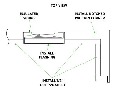
Because insulated siding is approximately 1-1/4" thick, you'll need to pack out trim boards to create a pocket for the siding.
