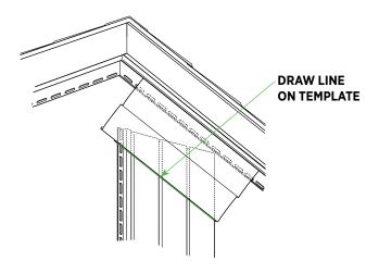
• Make a pattern for end cuts along the gable using two pieces of scrap siding. Lock one piece into the vertical strip at the center of the wall. Hold the edge of the other piece against and in line with the roof line. Mark the slope on the vertical piece and cut along that line. Use it as a template to mark and cut the ends of all other panels required for this side of the gable end. Make another pattern for the other side of the gable.
