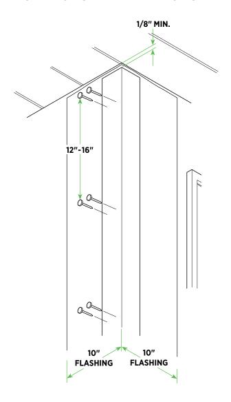
**Note:** A weather-resistive barrier must be applied before PVC trim is installed.
