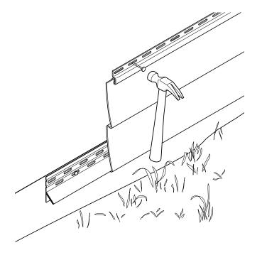
**Note:** A 6" minimum clearance should be given between ground and bottom of the first row. If there is a wave in the wall, use shims to straighten out the wall. This will help to smooth out uneven surfaces.
