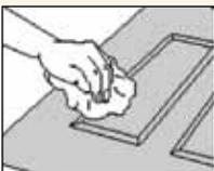
Steel doors should be wiped clean with a solvent such as mineral spirits. Allow the cleaning solvent to dry completely – until there is no residual odor. Once wiped clean, the door must be lightly sanded with a 220-grit sandpaper. After sanding, the door must be washed with a mild detergent in warm soapy water, rinsed and then dried.
