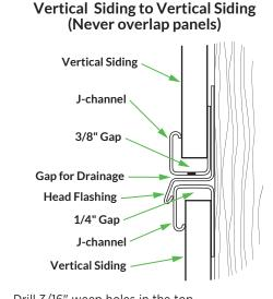
Drill 3/16" weep holes in the top J-channel no more than 24" apart.
