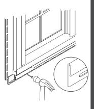
Required: install utility/under sill trim when the top nail hem has been removed, i.e., under the window and on the top course under an eave.
