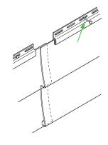
At panel overlaps, always fasten at least 3 nail slots from the overlaps. This will help with the lap appearance.
