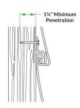
Fasteners must penetrate a nailable surface by 11/4".
