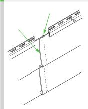
Use factory-over-factory laps to ensure proper movement of the panels.
