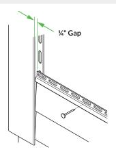
Leave a ¼" gap at all stops when the outdoor temperature is over 40°, and a minimum of ¾" gap when below 40°.
