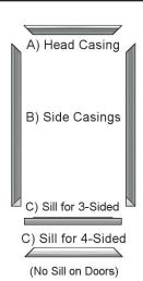
**1d) (Required)** Seal the accessory grooves. Apply a continuous bead of sealant along the length of the accessory groove before applying each piece of casing.
