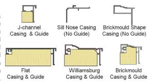
length but have a pre-cut miter on one end. Kits with rough length casing pieces also include a wood guide block (shown in illustration above) to assist in holding the casings in the proper orientation on your saw to ensure accurate cuts. Not all casing profiles come with guide blocks. Fasteners are included in all kits. Familiarize yourself with the pieces shown at bottom right before you begin.
