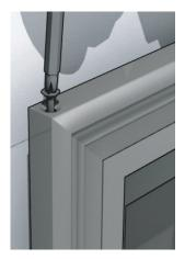
**1h) (Required)** Install the sill casing. Snap the sill casing into the accessory groove on the bottom of the window. For Sill Nose casings, fasten the sill casing to the side casings using an included #6 x 1½" Flat - head screw through the underside of the sill casing, being sure that it engages the screw boss in the side casings. For 4-sided casings, repeat the head casing process on the sill.
