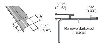
overall length and cut straight cut on the opposite end. To determine the overall length, first measure the unit dimension of the combination, then add the appropriate value for your casing from the "Sill Casing Lengths" table below. After cutting the sill nose to length, repeat the notching on the opposite end.
